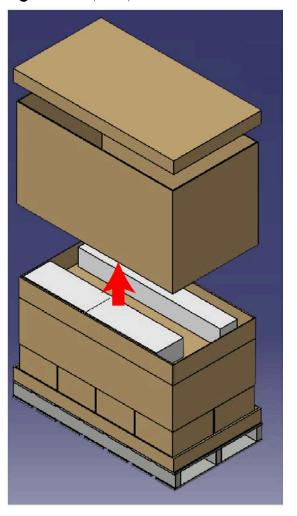
Figure 7: Top Cap and Sleeve Removal
