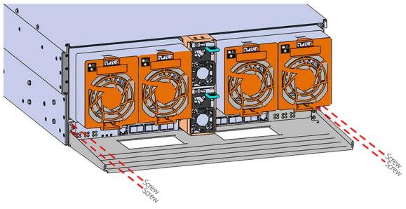
**Step 5:** Set the vertical rack rail depth to between 32" and 36".
