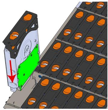
Figure 44: Installing a Drive Assembly
