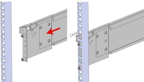
Figure 17: Front Rail Release Clip Operation
