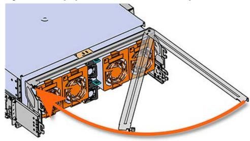
Figure 33: Swinging Motion of Crossbar to Locking Position
