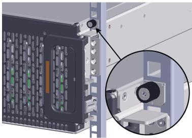
**Step 18:** Now that the chassis is installed, test the installation by sliding the enclosure in and out of the rack a minimum of three times. If the enclosure binds, catches, or displays any incorrect motion or behavior repeat the installation.
