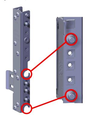
Figure 19: Spacer Bracket Orientation
