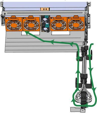
Figure 40: Connected Cable Routing
