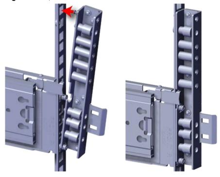
**b.** Slide the nut plate down over the mounting pin on the back of the spacer bracket.
