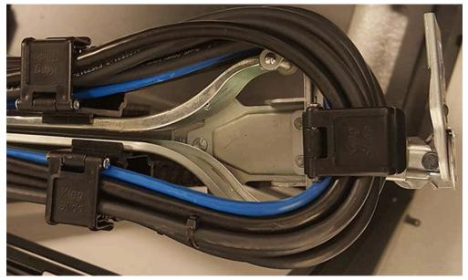
At the end of the CMA where the cables exit, use a cable tie to bundle the cables together. Make sure the cables are bending and not twisting.
