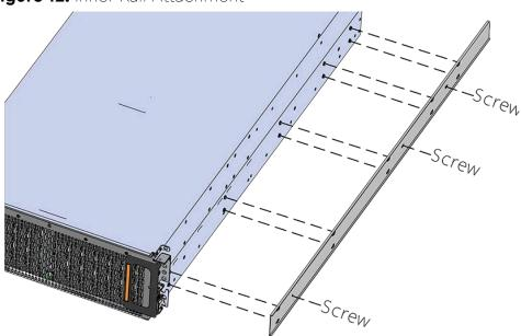
Figure 12: Inner Rail Attachment
