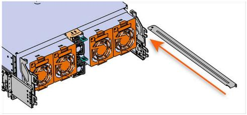
**b.** Insert the peg on the underside of the crossbar into the slot on the CMA mounting bracket.
