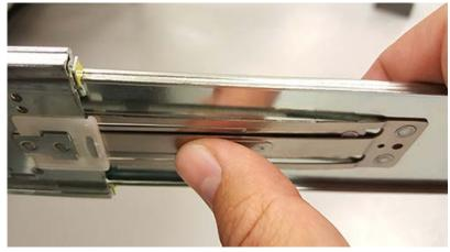
**e.** As the chassis is slid into the rack, position one installer at the rear of the rack to ensure that the pegs on the sides of the cover will slide correctly into the rear cover alignment brackets on both sides of the rack. If the chassis does not install smoothly or snags, check that the rear cover alignment brackets are not interfering with the chassis sidewalls, and try again.
