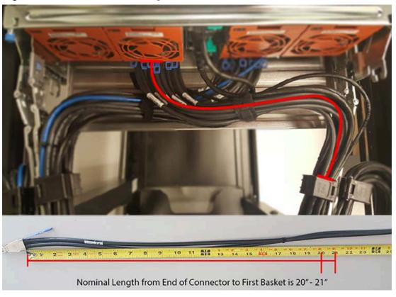
Figure 48: Nominal Cable Length at Connectors
