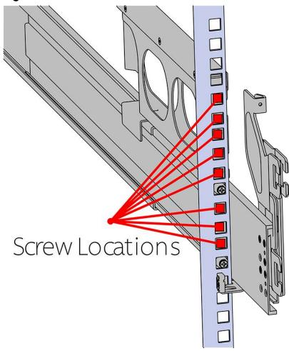
Figure 25: Screw Installation Location
