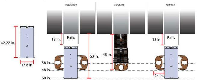
Figure 5: Installation, Servicing, and Removal
