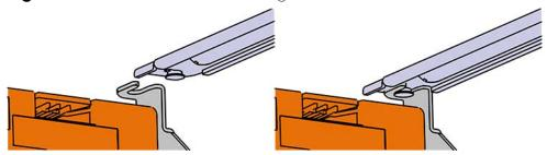
**c.** Swing the crossbar so that the thumbscrew lines up with the mounting hole on the opposite side of the enclosure.
