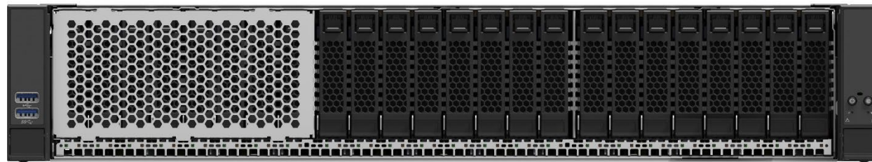
Figure 15. Intel® Server System M20NTP2UR 16-Drive Configuration (with Accessory Kit Options)
