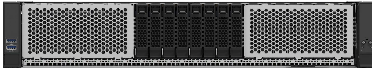
Figure 14. Intel® Server System M20NTP2UR 8-Drive Configuration (Default)
