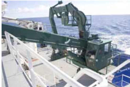
15T fixed boom crane, 40 feet long, on cargo vessel
