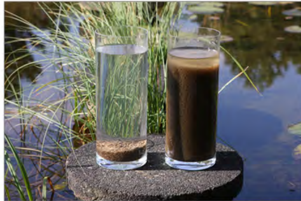
Comparative settleability of AGS granules (left) and activated sludge (right) after 5 minutes
