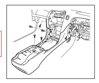
2. Remove the shift lock control ECU sub–assembly, found on the driver's side of the shift assembly.
