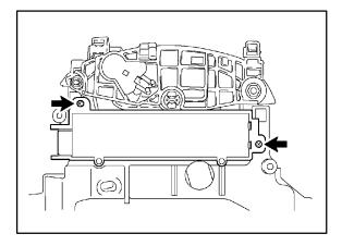
3. Remove the original shift lever anti–rattle cushion and replace with the new part, as shown in the illustrations.
