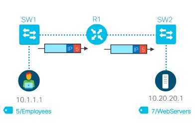
SGT carried inline in the data traffic. Methods include, SGT over:
