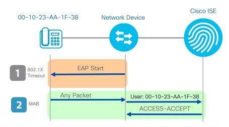
MAB requires a MAC address database | ISE can build this database dynamically with profiling
