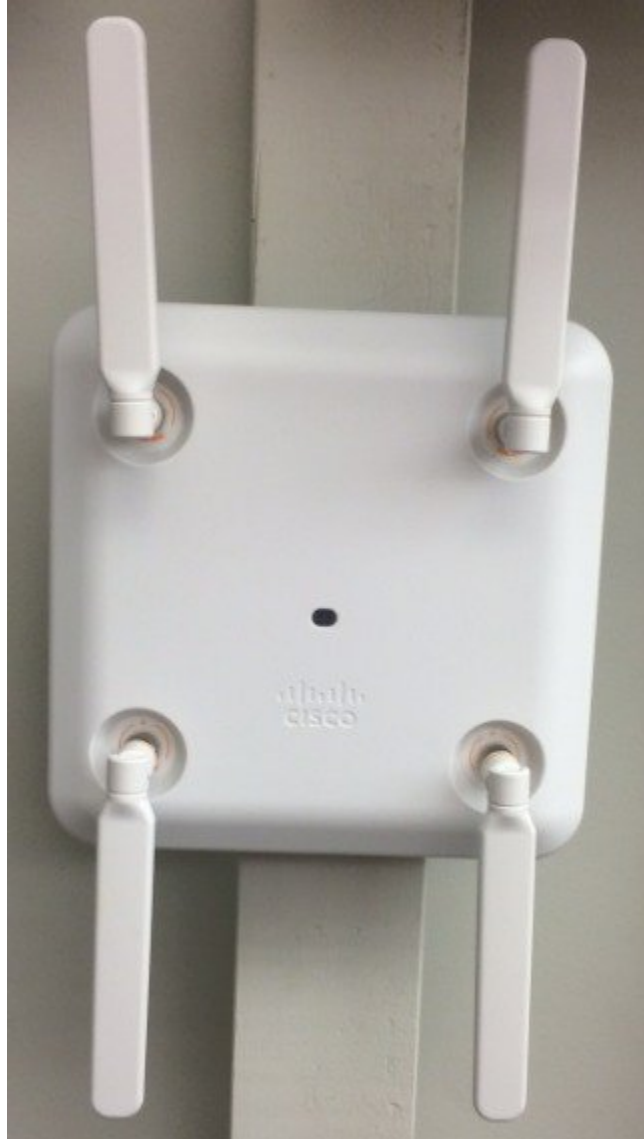
Figure 10: Avoid wall mounting units with internal antennas
