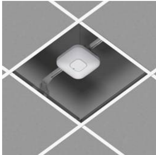
Figure 15: Oberon Model 1045- Above ceiling hanger kit - this includes a hanger bar and wire, and a light pipe that can be pressed through the ceiling tile so you can see the status LED from below, without lifting ceiling tile
