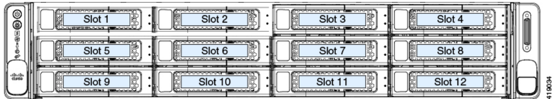
Figure 18: Large Form-Factor Drive (12-Drive) Version, Drive Bay Numbering
