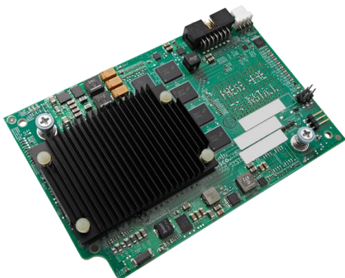
Figure 6 Cisco UCS Virtual Interface Card (VIC) 1340
