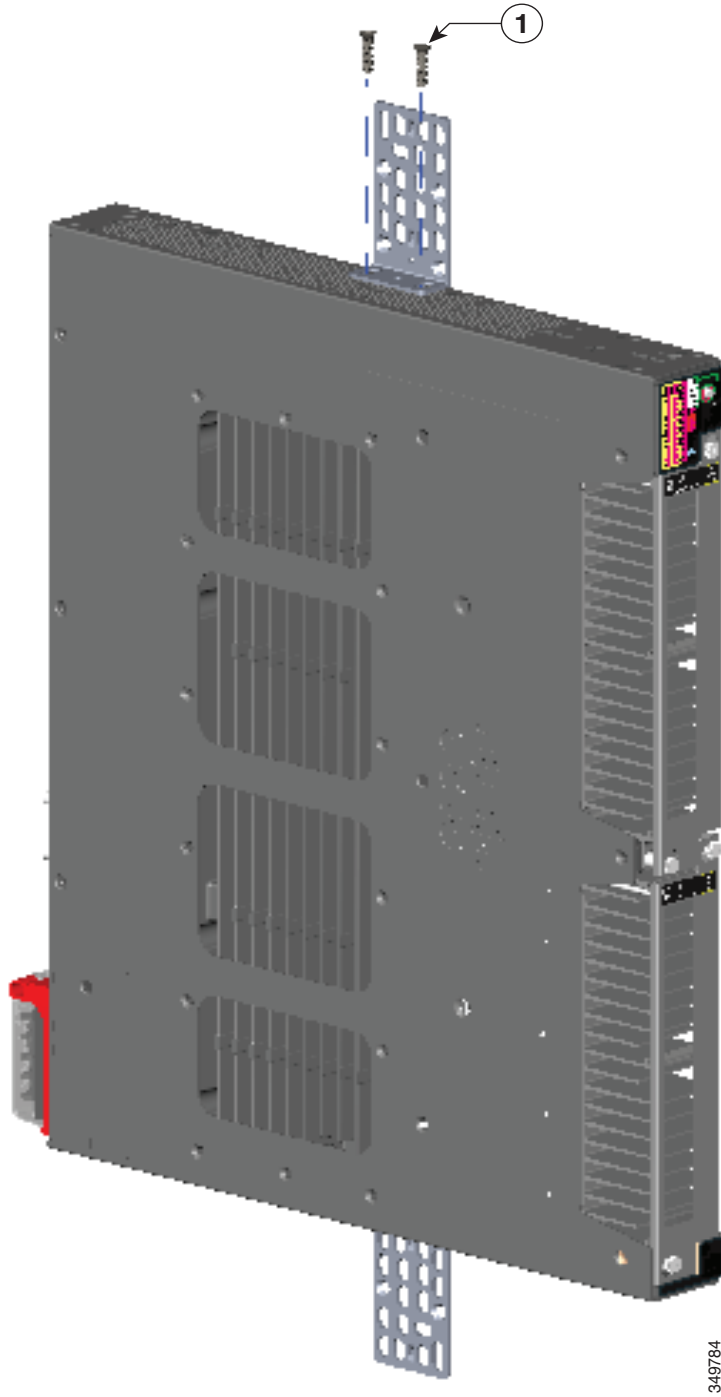
Figure 15 Attaching 19-inch Rack Brackets
