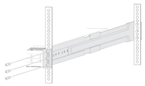
d) Tighten the 10-32 screws to 20 in-lb (2.26 N·m) or tighten the 12-24 screws to 30 in-lb (3.39 N·m).
