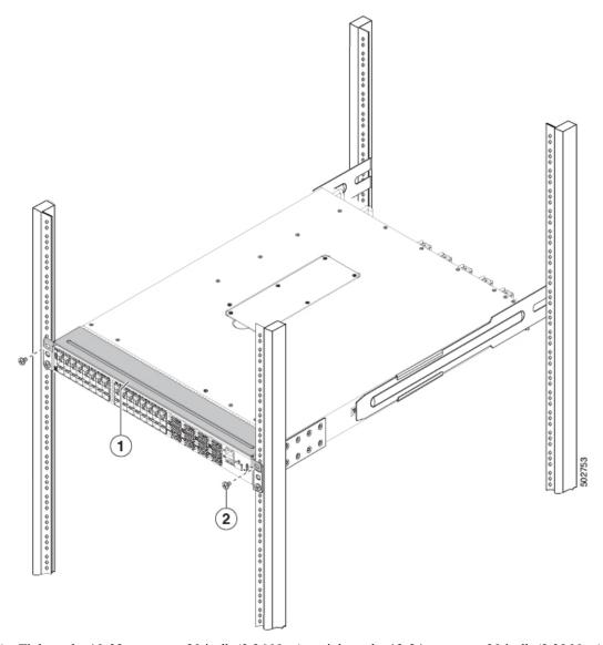
c) Tighten the 10-32 screws to 20 in-lb (2.26 N·m) or tighten the 12-24 screws to 30 in-lb (3.39 N·m).
