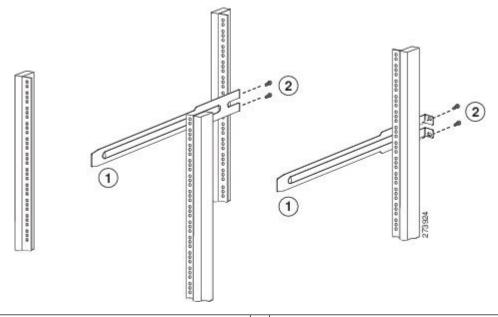
Slider rail with screw holes aligned to screw holes in rack
