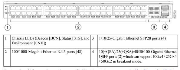
The following figure shows the hardware features seen from the port side of the chassis.
