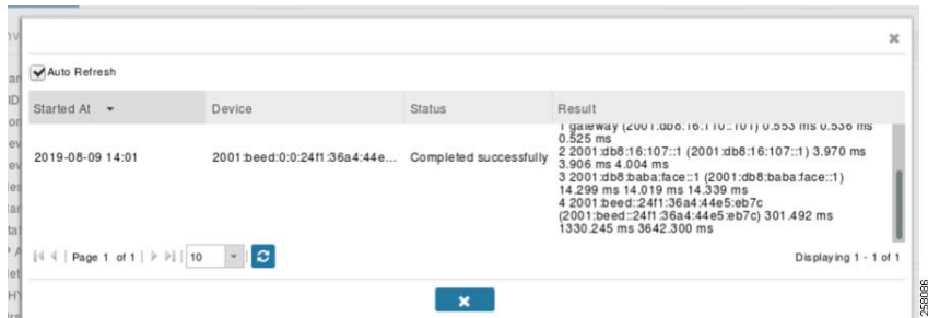
Figure 180 Traceroute from FND to CGE
