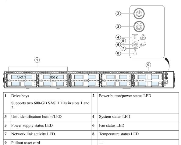
The following figure shows the front panel features and disk-drive configuration for the ESA C695 and C695F. See Front Panel LEDs, on page 8 for a description of the LEDs.
