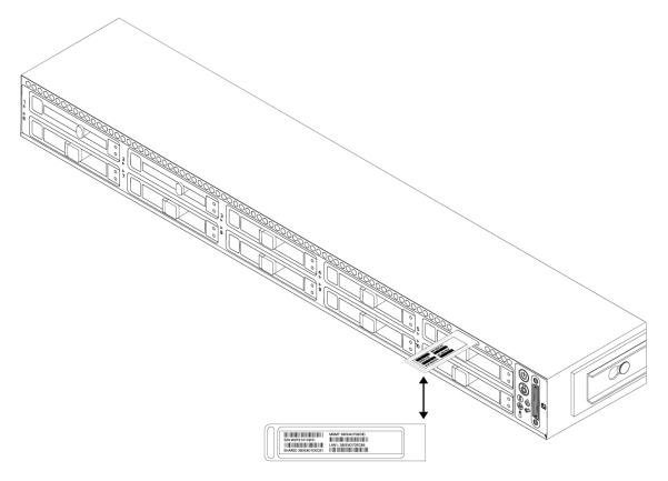
The serial number is also on the label on the cover of the chassis as shown in the following figure.
