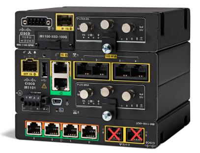
In this configuration, the ethernet ports on the IRM-1100-4A2T will not function. The serial ports have full functionality.
