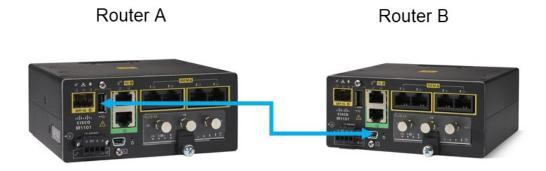
The blue line above is a USB 2.0 Type A to USB 2.0 mini USB Type B cable. Refer to this topology for the following configuration.
