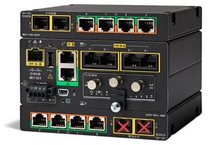
In this configuration, the IRM-1100-4A2T mounted on the Expansion side, or top, has full functionality. The Ethernet ports on the IRM-1100-4A2T mounted on the Compute side, or bottom, will not function.
