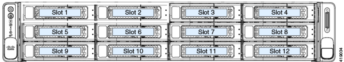
Figure 20: Front Drive Bay Numbering, LFF Versions
