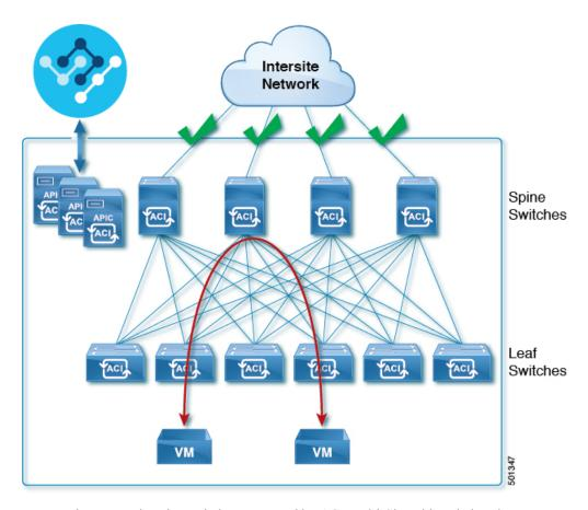
You can choose to mix spine switches supported by ACI Multi-Site with switches that are not supported within the same Cisco APIC fabric but only the supported switches can connect to the intersite network as shown in the following figure.
