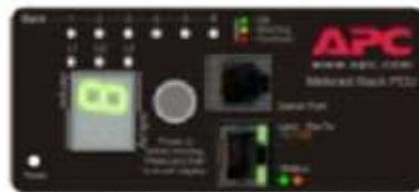
User interface: On-board metering display and network connections
