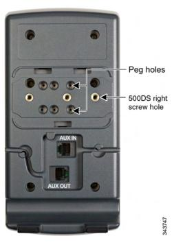
STEP 7 Using an attachment arm screw, secure the attachment arm to the Cisco SPA500DS.
