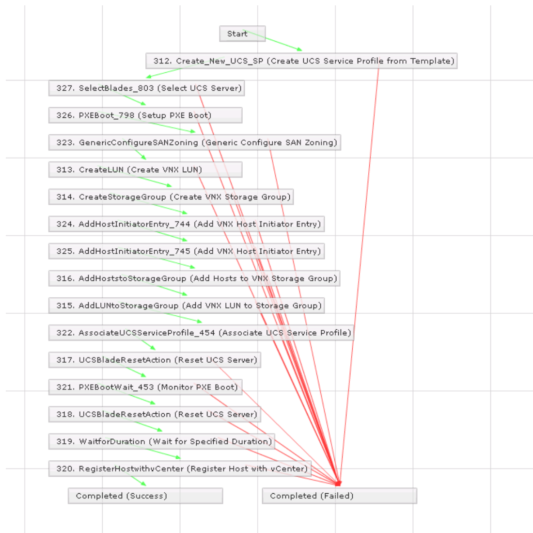
Figure 31 DaaS Workflow Diagram for Installing ESXi on Cisco UCS B200 M3 Servers
