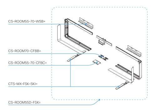
If you have a Room 55 Dual that is mounted on a floor stand, you have to order the following parts in order to change to the wall mounted option:
