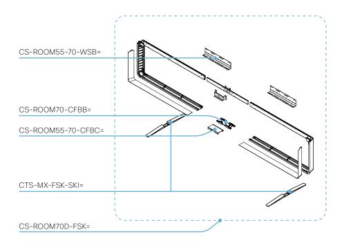
If you have a Room 70 Dual that is mounted on a floor stand, you have to order the following parts in order to change to the wall mounted option:
