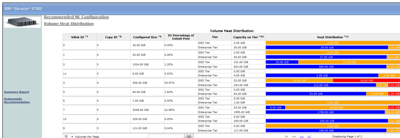
Figure 14-1 The Volume Heat Distribution that is found by using the STAT tool
