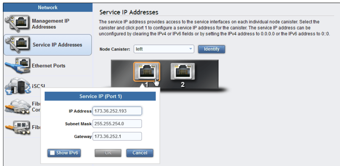
Figure 7-11 Set the service IP for port 1
