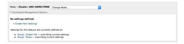
This is exactly what I'd like to see. Realize that nearly all of the remaining portion of the config is at the Cluster level. Your webUI will be at the Cluster level nearly all the time and if you then Navigate to Network > DNS (while in cluster mode), you will realize that there are no DNS settings at the mode and you will go to each Group mode to make the DNS changes — which is what we want to do because the ESA appliances are installed in different Data Centers.
