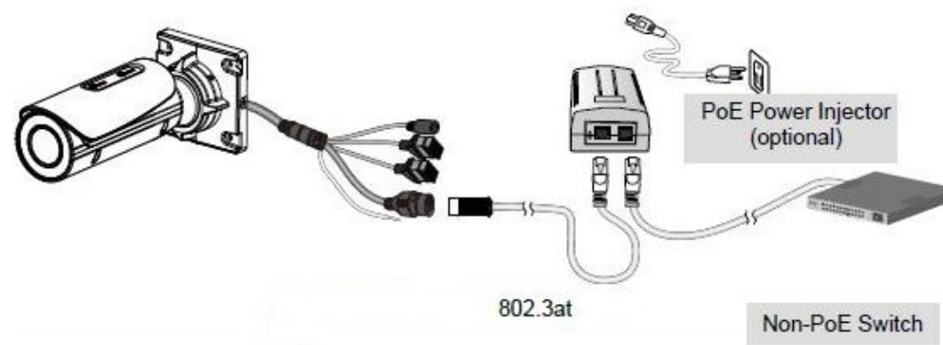
Figure 1-3 Connecting the Camera to a Non-PoE Switch
