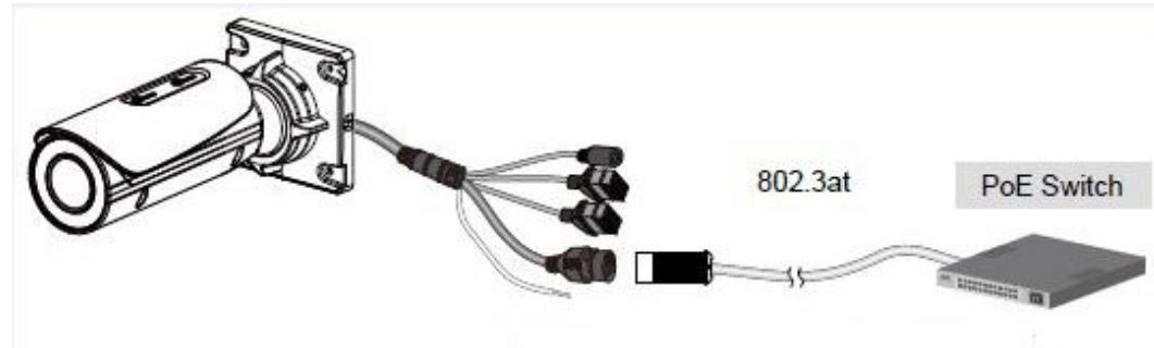
Figure 1-2 Connecting the Camera to a PoE-Enabled Switch
