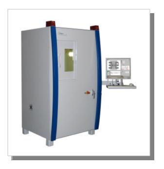
Powered by user-friendly FEINFOCUS Graphical User Interface (FGUI) software, the COUGAR-VXP includes a microfocus X-ray tube up to 160 Kv, standard 5-axes manipulator with Auto Isocentric Motion (AIM) Technology<sup>™</sup> for oblique viewing, CNC Capabilities, FEINFOCUS HDX-ray<sup>™</sup> real-time 16-bit image processing, CMOS digital flat panel detector, and a hardware-driven anti-collision system. The system provides feature recognition down
