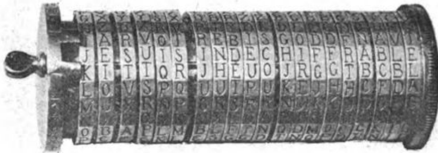
Bazeries cylinder. Photo courtesy of Étienne Bazeries. The cylinder is set to encipher the phrase “I am indecipherable.”
