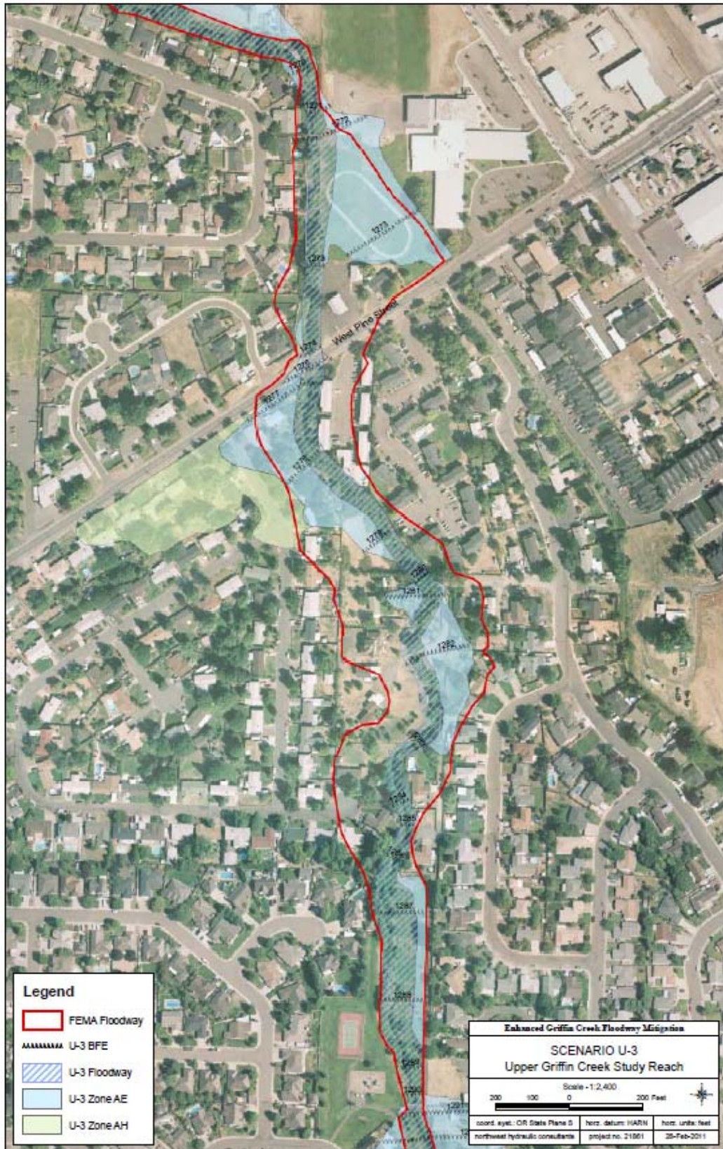
Figure 6.12 Griffin Creek Mitigation: Upper Reach Results
