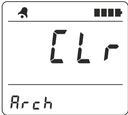
Figure 30 – LCD of the radiometer (the submode of measurement results clearing stored in the nonvolatile memory)
