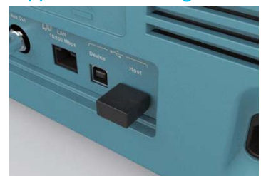
Wi-Fi adapters are configured through integrated setup menus and support seamless wireless communications
