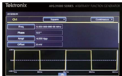
With InstaView on AFG31000 turned off. Due to an impedance mismatch, the AFG display shows a different waveform from the one observed at the DUT.
