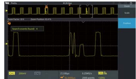
Search and Mark features for easy identification of events that occur in the acquired waveform
