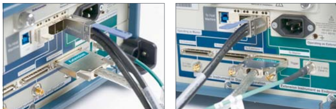
UltraSync connection on instrument with Master and Extension role
