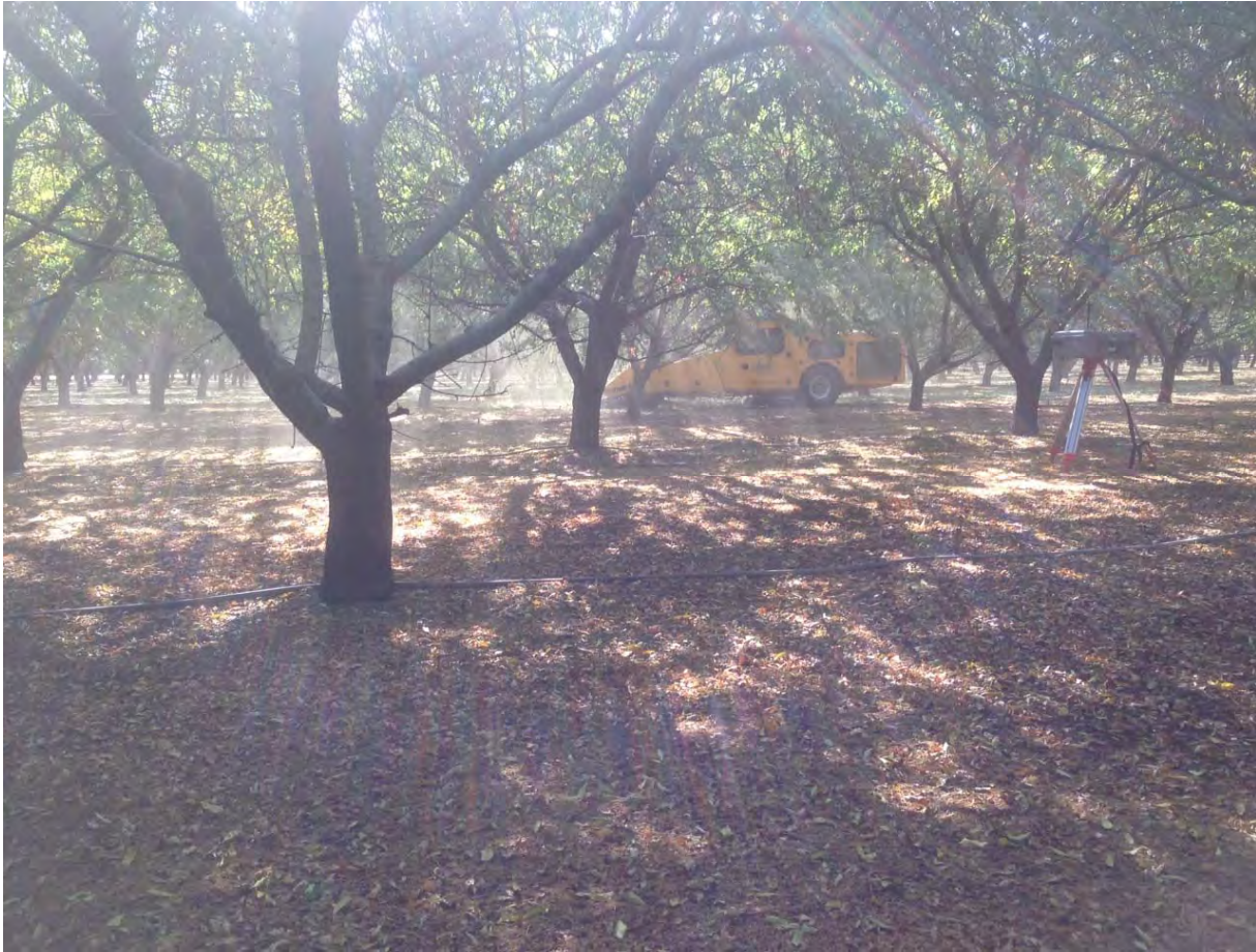
Figure 6. Deployed dust monitor during the shake process of the first year.
