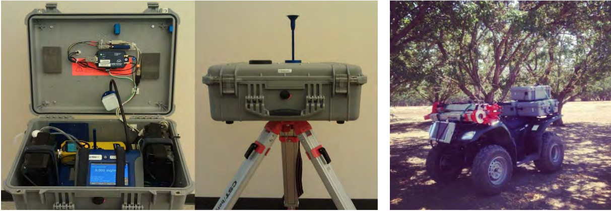
Figure 4. Dust emission monitor (laser photometer) and data logger in ruggedized case (left) and mounted on ATV at field site (right).
