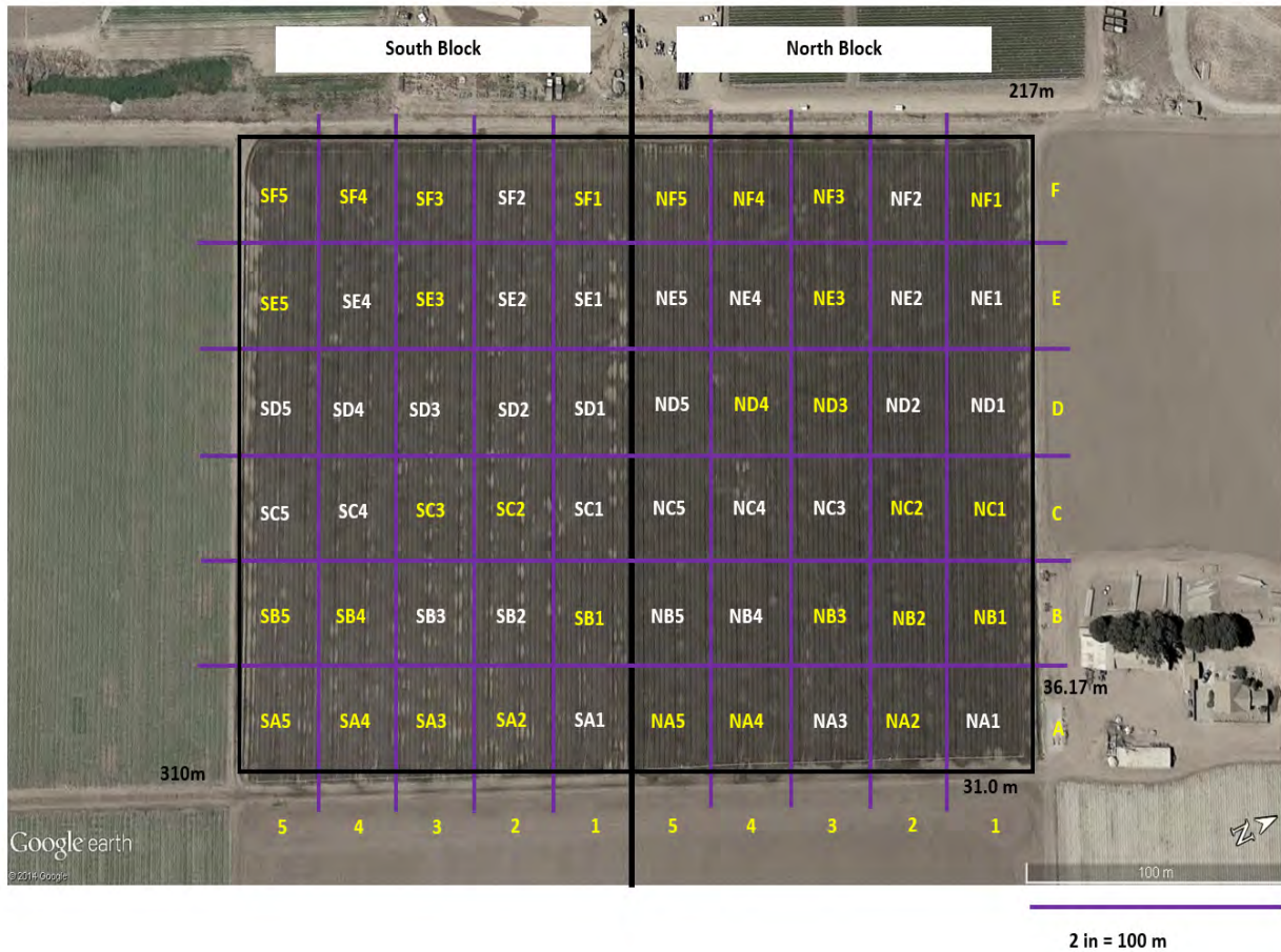
Figure 2. North and South treatment blocks gridded into 30 squares each. Lysimeters were placed within each of the gridded squares.
