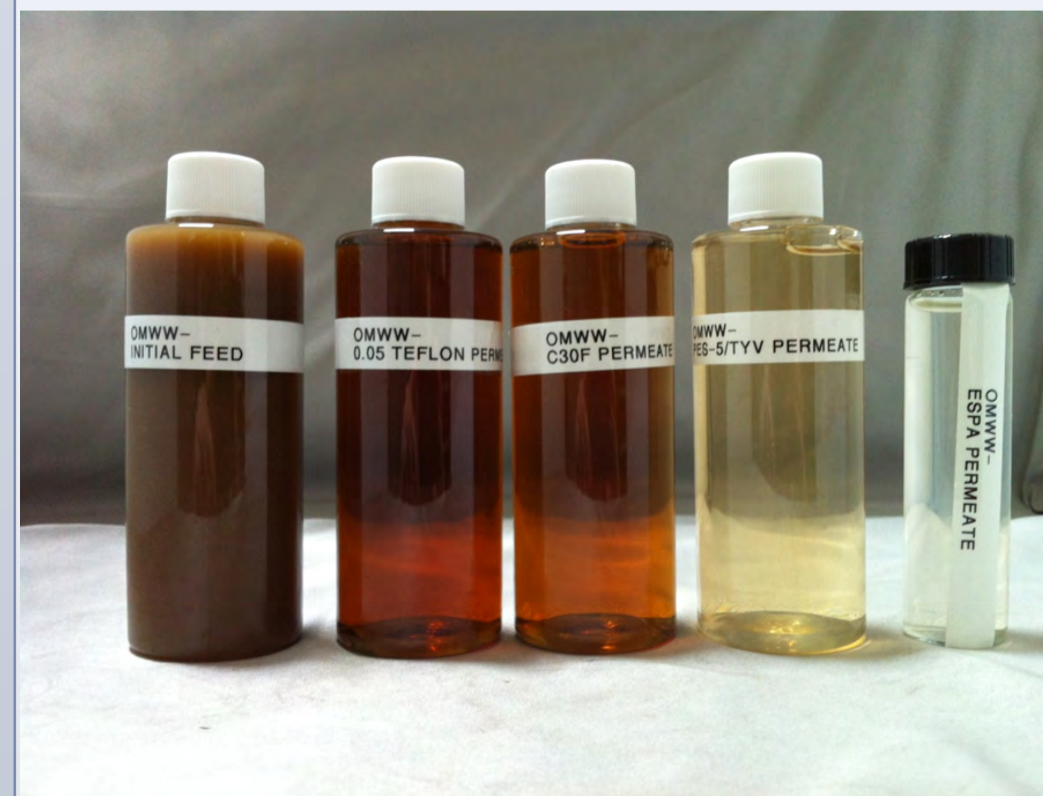
Fig.1 Membrane selection result, left to right: Initial Feed, 0.05 Teflon, C-30F, PES-5, ESPA
