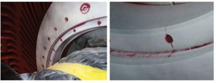
37. Red-dye confirmation of cracks is shown at left and right
