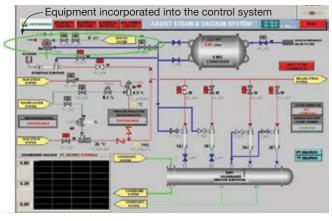
**2. Equipment incorporated into the DCS** to provide tighter control over vacuum-raising is highlighted in the diagram
