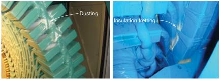
12. Endwinding vibration is a major cause of dust generation
