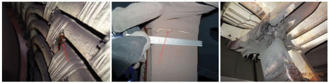
**11. Overheat damage** shown at left and in center led to the connection-ring failure at right 12
