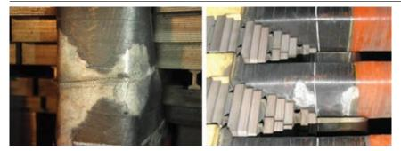
**16. OCP** (outer corona protection) erosion is shown on bars (left) and at core ends (right)
