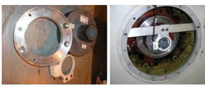
17. EFREM system components are shown individually at left, assembled at right
