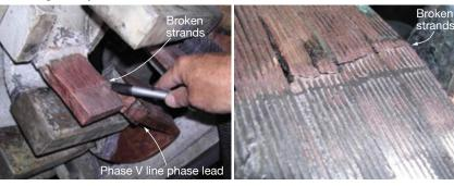
27. Cracked strands at the top of the pen at left are shown in detail at right
