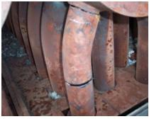
**4. Several tubes failed** in the HRSG reheater bundle next to the outer wall of the unit
