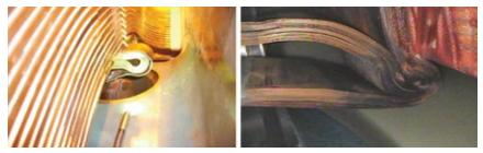
**31. Broken J-straps:** Complete J-strap separation from main terminal stud is at left; a deformed, collapsed J-strap is at right
