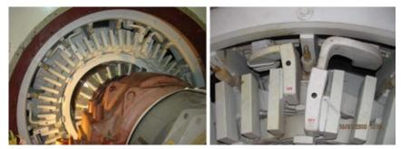
**25. Original end winding** showing phase-bar blocking design is at left; closeup at right. Supports use rope ties and conforming felt layer
