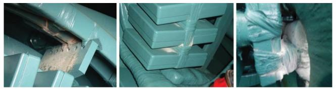
**34.** Several cases of endwinding and connection-ring vibration were found during generator inspections. At left and right is connection-ring dusting on blocks/ties, in center is greasing on series loop blocks
