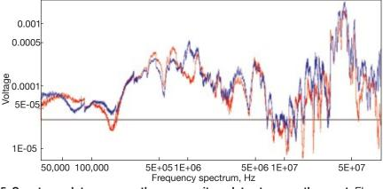
5. Spectrum plot compares the same unit on dates two months apart. Electrical activity increased between the first (red) and second (blue) scans
