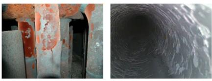
6. Oxide exfoliation of tube external surface is clearly visible at left, internal surface (via borescope exam) at right. Exfoliation is an indicator of overheating
