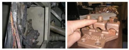
**33. Failed exciter lead connection** at left was corrected with an upgraded connector (right)
