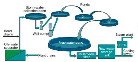
2. Network of ponds collects rain and snow-melt runoff for plant makeup
