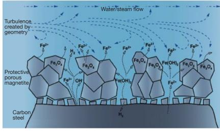
**2. Two-phase FAC** (steam and water) is a consequence of a flow-accelerated increase in mass transfer of dissolving and reacting species at a high-flow or highly turbulent location
