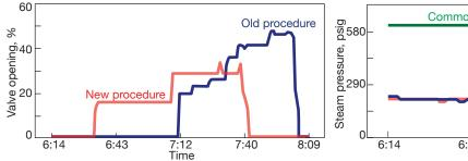
**2. Reduction in steam venting** during startup saved a significant amount of water
