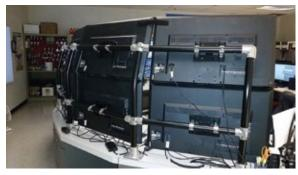
**1. Custom structure** made of conventional components supports two tiers of monitors
