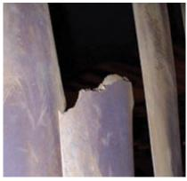
19. LP turbine L-0 blade failure
