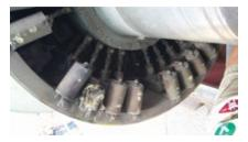
**29. Diode wheels** suffered significant damage. All fuses on the inboard wheel were open
