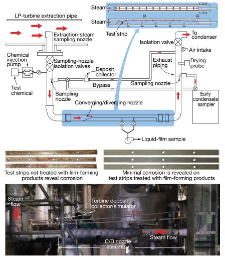
**1. Test loop** simulates LP-turbine expansion using a converging/diverging (C/D) nozzle (top). Results indicate filming amines and products can offer significant corrosion protection against contaminants as shown by the two sets of test strips (middle) . Photo of the test setup is at the bottom
