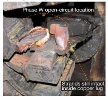
**26. Failed joint** reveals extensive burn damage
