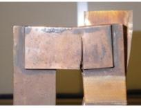
22. Severe tear in pole-to-pole connector
