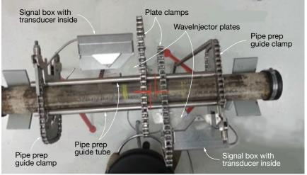
22. WaveInjector® ultrasonic detection can pinpoint water in drain lines
