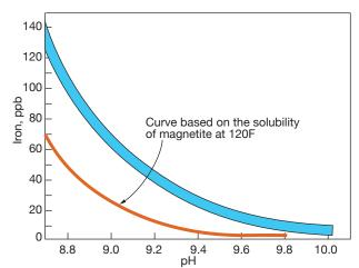
1. Dooley/Aspden relationship, important to ACC operation, graphs the relationship between pH and total iron. Note that ammonia was used exclusively for pH control in this case: iron levels were measured at the condensate-pump discharge. Data for iron solubility are attributed to Piero Sturla of ENEL's Piacenza Laboratory (1973)
