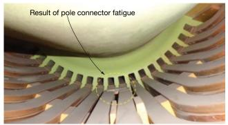
19. Result of field-winding pole connector fatigue is clearly in evidence
