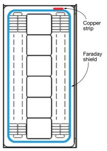
**2. Faraday shield** consists of a semi-conductive tape (blue) around the copper strands. This layer of semi-conductive tape helps create an even ground wall across the tube to copper. A copper strip connects from the semi-conductive layer to a single strand in the copper, ensuring a single path to ground
