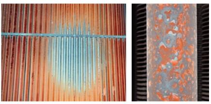
5. Overheat zone is clearly visible on panel at left; impact of overheat on tube internal surface is at right
