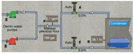
3. Monitoring of condenser makeup flow warns plant personnel of leaks
