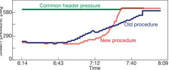
**3. Steam-pressure** ramped to header pressure faster using the new startup procedure
