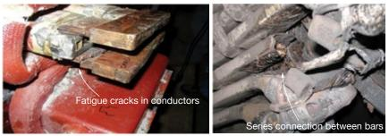
**13. Failures resulting from endwinding vibration** can cause considerable collateral damage
