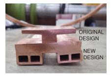
24. New pole connector design is shown below old design
