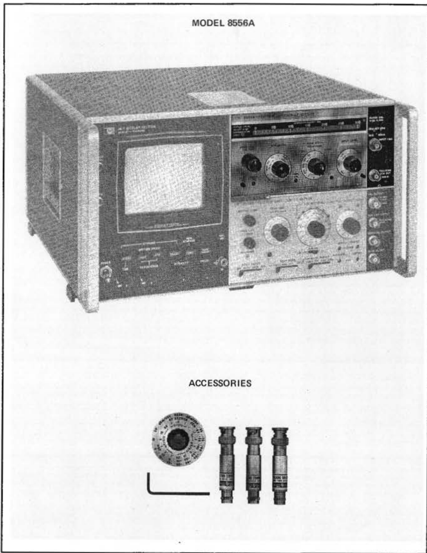
Figure 1-1. Model 8556A Spectrum Analyzer LF Section with 8552B IF Section and 141T Display Section
