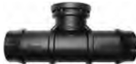
800-02350 25MM BARBED X 1/2" BSP FEMALE THREADED TEE
