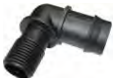
800-02368 25MM BARBED X 1/2" BSP MALE THREADED ELBOW
