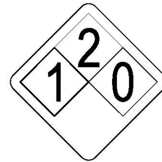
ALERTING SIGN (FOR DIESEL FUEL)
