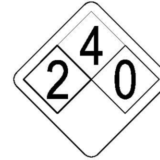
ALERTING SIGN (FOR PROPANE)
