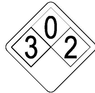
ALERTING SIGN (FOR CELL SITE BATTERIES)
