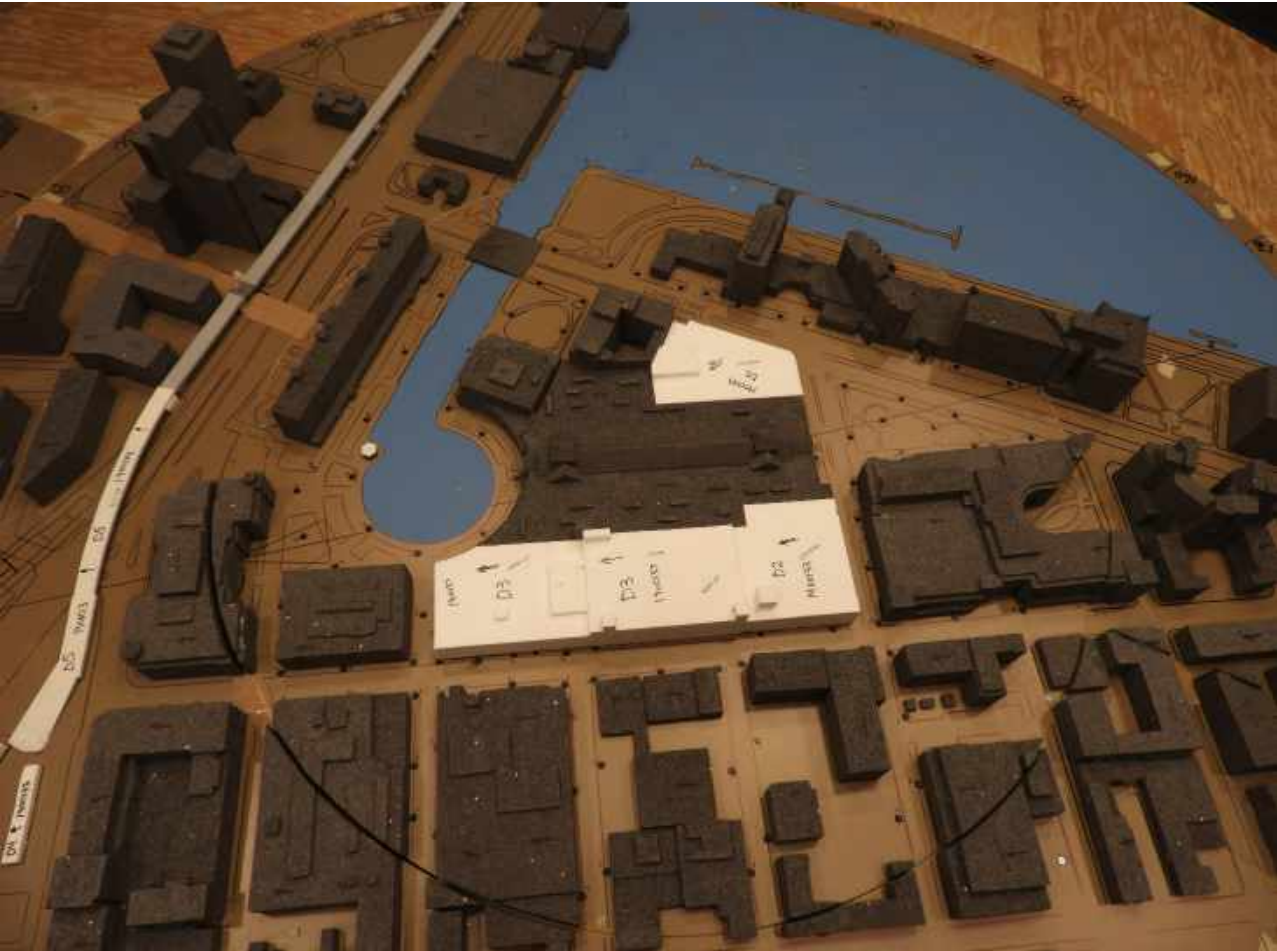
Image 2A: Wind Tunnel Study Model - No Build Configuration
