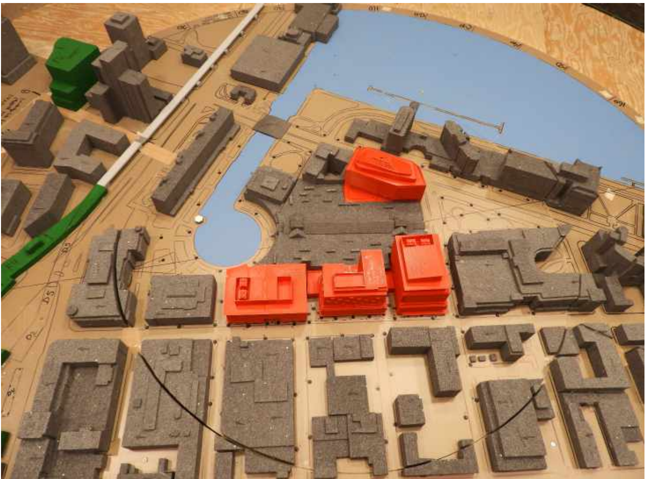
Image 2C: Wind Tunnel Study Model - Full Build Configuration
