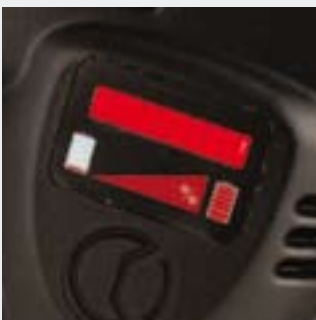
Battery condition display
