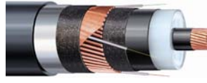
Aluminium laminated sheath with Copper wire screen and integrated fibres for temperature sensing
