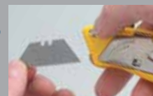
Push button to use other side of current blade.
