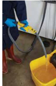
Remote high flow bucket/autoscrubber fill gun.
