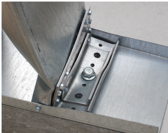
RCKW assembly test with member failure.
