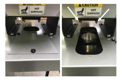
Slide the <u>cast aluminum collection</u> <u>hopper</u> onto the threaded rods of the vacuum chamber fill valve assembly.
