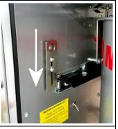
Install the air lines. Rotate the locking ring fully clockwise to secure the air connection.
