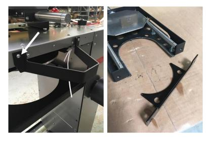
Insert the <u>upper vacuum slide gate</u> <u>assembly</u> into the groove of the mounting collar on the vacuum chamber tank head.
