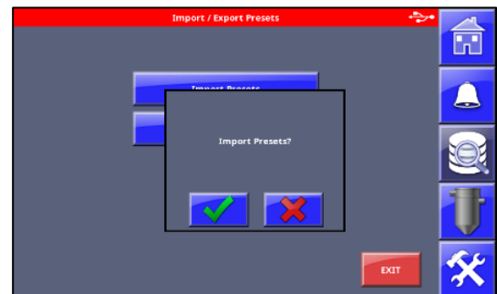
Plug in USB with new material preset added to .CSV file and press the 'Import Presets' button.
