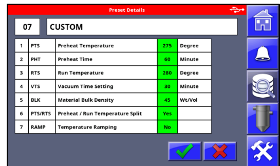
The parameter values in the 'Preset Details' screen will mimic what was inputted into the .CSV file.
