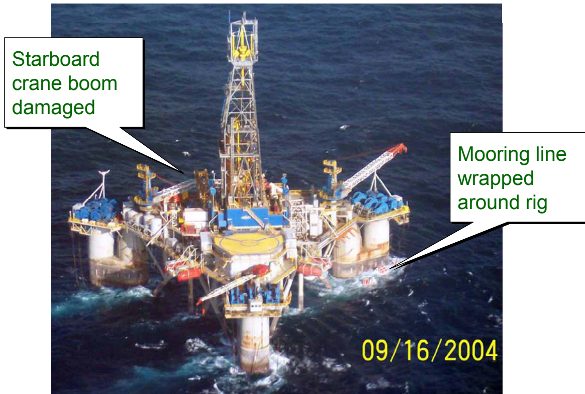
Figure 14: Noble Jim Thompson with damages noted.
