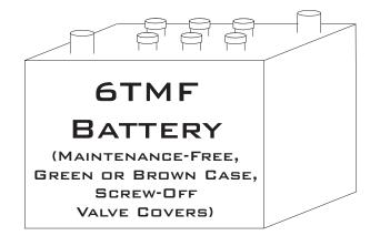
CEN N3215B Regulator Setpoint MUST be set to Position #2 on underside of regulator for 6TMF, 6TLFP, or **6TLMF** batteries
