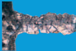
Severe corrosion. The grid becomes brittle.
