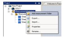
From the context menu of a measurement page, the folder can be renamed and deleted. It also allows the creation of measurement pages.
