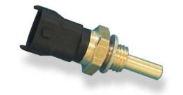
The NTC sensing element has a negative temperature coefficient. This means, that with increasing temperature the conductivity rises. The sensing element of the temperature sensor is made of semiconducting heavy metal oxide and oxidized mixed crystals, which are equipped with a protective housing.
