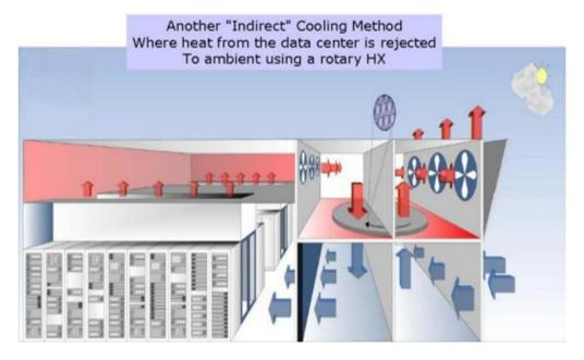
Theory behind rotary heat exchanger technology
