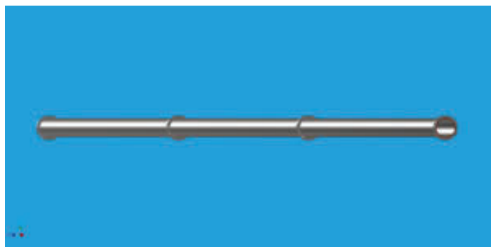
Figure 1. (top) full assembly of the temporary beam pipes Figure 2. (bottom) the three sections of stainless steel beam pipes
