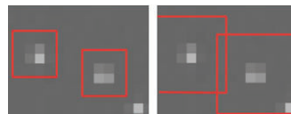
Figure 6. Example of two separate footprints with a grow factor of 1 (left), and the footprints merging into one footprint when a grow factor of 3 is applied (see figure 7).
