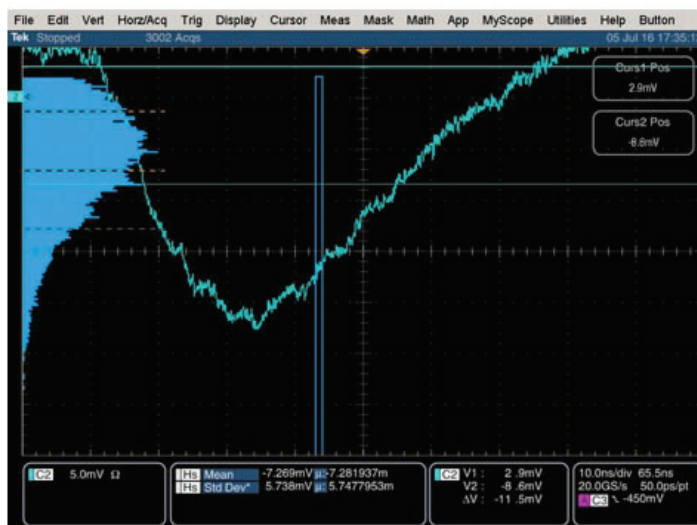
Fig. (29) Image of the 15um SiPM's initial output pulses after exposure to 1 MRad gamma irradiation.
