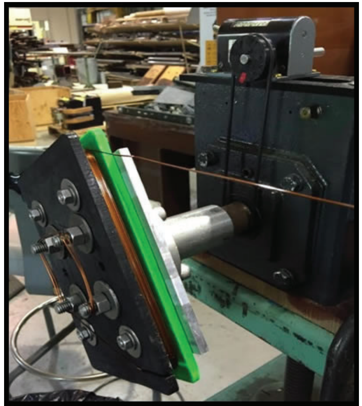
Figure 4: Pictured to the left is the entire assembly for our coil production process. Visible here are various components including the winding machine, winding fixture, stress relief plate, copper wire, and turn counter (the details of which will be discussed in the next section).
