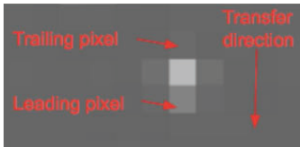
Figure 4. Example of trailing and leading pixels in x-ray hit on CCD.
