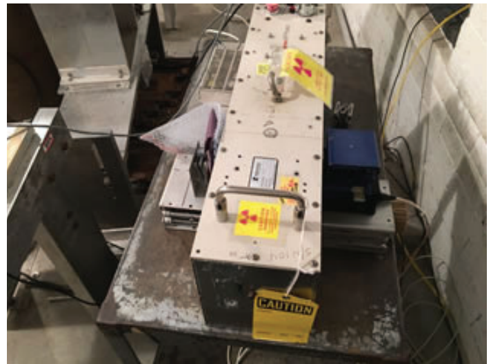
Fig. (6) The set-up for SiPMs irradiated at BNL's Solid State Gamma Irradiation Facility (SSGRIF) using a 14MeV neutron generator.
