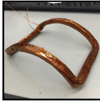
Figures 6 and 7: The images above show a sample of one of our bent coils and the mold that it fits into. Like this sample, all coils were consistently bent to match the radius and general shape of their corresponding coil form.
