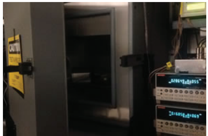
Fig. (8) SiPMs Saturation curves were measured using a pulsed LED and a charge integrating ADC. This is the setup. (It will be)
