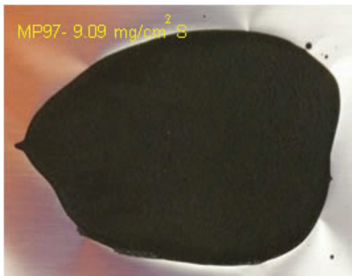
Figure 9. Electrodes of very high sulfur loadings achieved using MP97 as the carbon additive material only.
