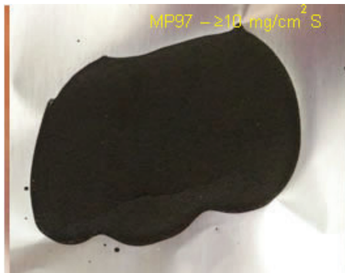
Figure 9. Electrodes of very high sulfur loadings achieved using MP97 as the carbon additive material only.
