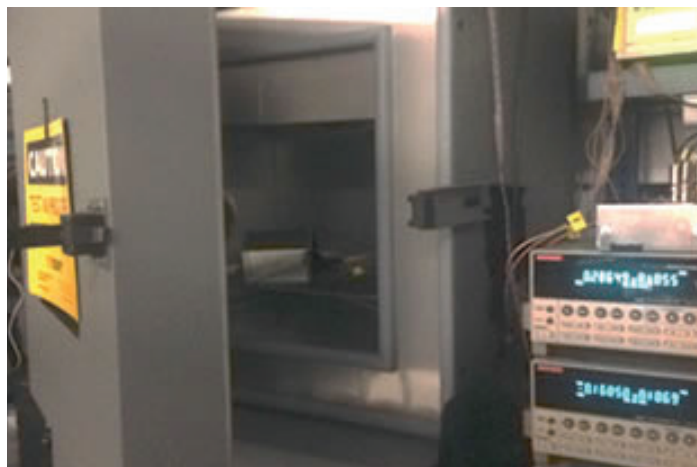
Fig. (7) SiPMs Dark Current measurements were taken using a Keithley K657 Picoammeter and a voltage source. The setup can be seen here with the SiPMs inside the light tight box.
