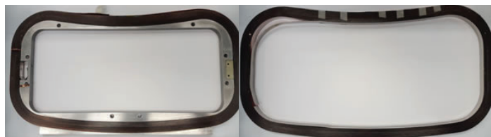
Figure 3: YBCO HTS dipole magnet coil with support structure (left) and YBCO HTS dipole magnet coil without support structure (right)
