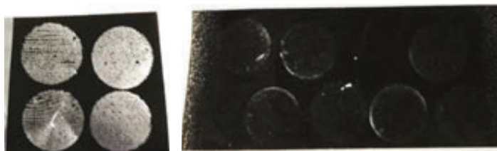
Figure 4. Electrodes of 1.3 mg/cm 2 sulfur loading after tape test, Ketjen Black (left) and MP97 (right).
