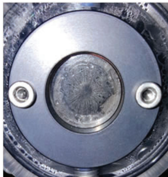
Fig. 4. Starburst pattern on the impactor of the PILS.
