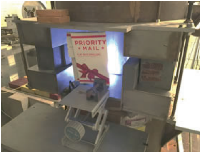
Fig. (5) The set-up for SiPMs irradiated at BNL's Solid State Gamma Irradiation Facility (SSGRIF) using a 60 Cobalt gamma source.
