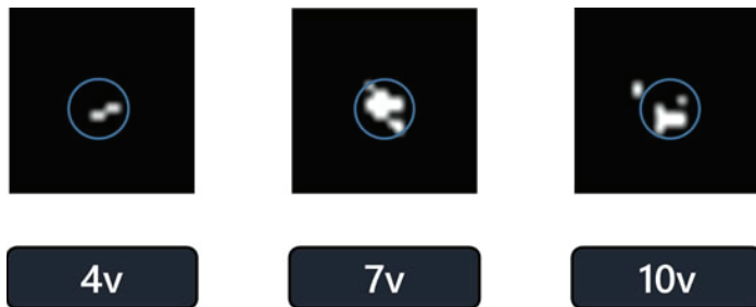
FIG. 3. Single frame hits corresponding to a specific LED voltage.
