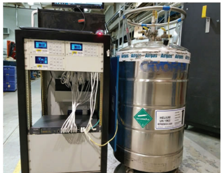
Figure 1 & 2: Figure 1 shows one of the 64 strain gages on the outer shell of the LARP test magnet. Figure 2 shows the chassis setup for the level probes. A cryostat filled with 60L of liquid helium is shown as it was used in for sensor calibration.
