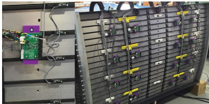
Figure 2: Outer HCal prototype, close up of the circuit board and the SiPMs
