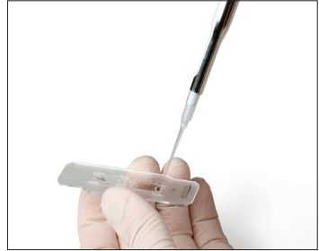
Fig. 9. Loading the counting slide.
