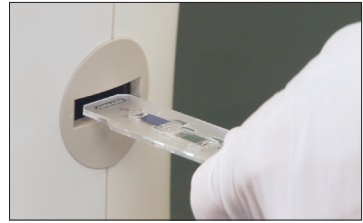
Fig. 10. Inserting the counting slide into the TC20 cell counter.
